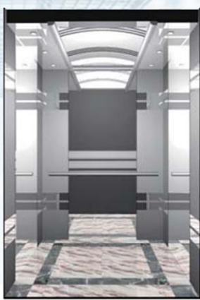
HL-809-3 Car ceiling: mirror stainless steel frame, tube light, transparent panel middle Car wall: mirror, hairline combination Handrail: HL-301F Floor: HL-728PVC
