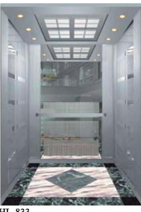
HL-833 Car ceiling: HL-462 hollow ivory acrylic pillars, gold tube light Car wall: 1: central panel: mirror, etching 2:auxiliary panel: hairline panel Handrail: HL-313F Floor: HL-727PVC
