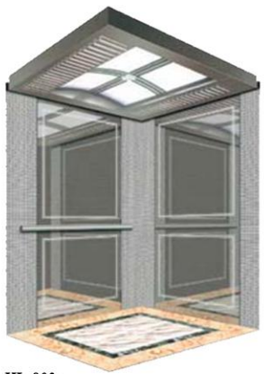
HL-803 Car ceiling: HL-420 rectangle hollow transparent lampstand on mirror stainless steel bottom panel, middle part-concave ivory transparent panel Car wall: 1.central panel: mirror, etching, hairline, irregularly-lined 2. auxiliary panel: mirror, etching Handrail: HL-301F Floor: HL-702PVC
