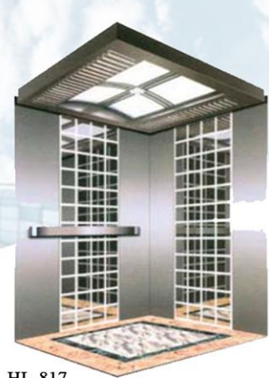
HL-817 Car ceiling: HL-420 rectangle hollow transparent lampstand on mirror stainless steel bottom panel, middle part—concave ivory transparent panel Car wall: 1.central panel: mirror, etching, hairline 2.auxiliary panel: hairline panel Handrail: HL-313F Floor: HL-702PVC
