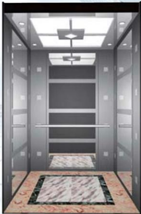
HL-809-2 Car ceiling: mirror stainless steel frame, tube light Car wall: hairline etching, mirror, hairline combination Handrail: HL-301F Floor: HL-702PVC
