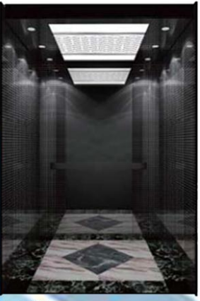
HL-808-18 Car ceiling: black titanium mirror stainless steel tube light, middle painted steel sheet Car wall: black titanium panel, black etching panel Handrail: black titanium hairline oblate handrail Floor: HL-727PVC
